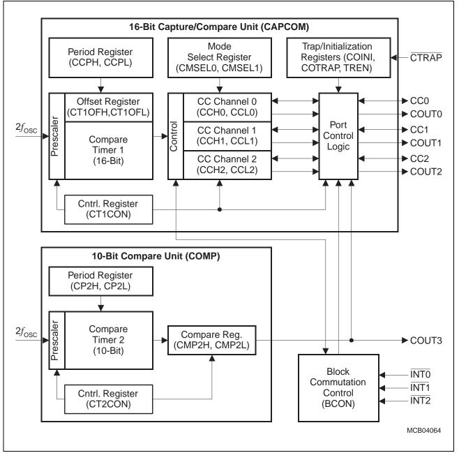
Figure 14 Block Diagram of the Capture/Compare Unit CCU
