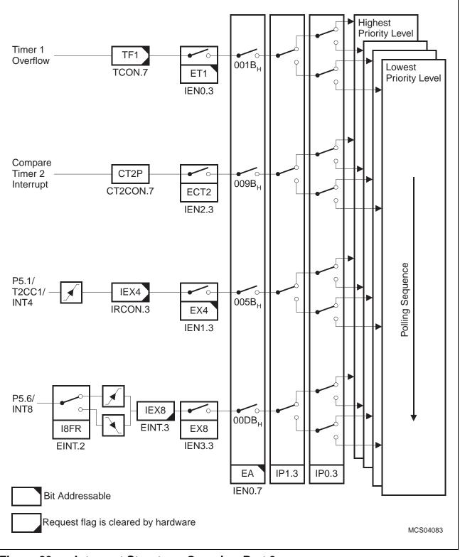
Figure 23 Interrupt Structure, Overview Part 3
