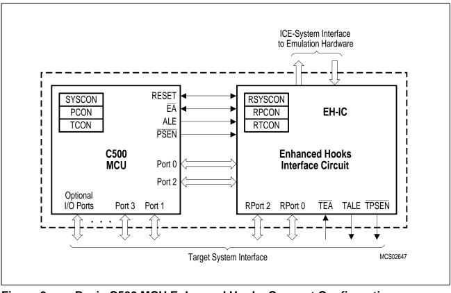
Figure 9 Basic C500 MCU Enhanced Hooks Concept Configuration
