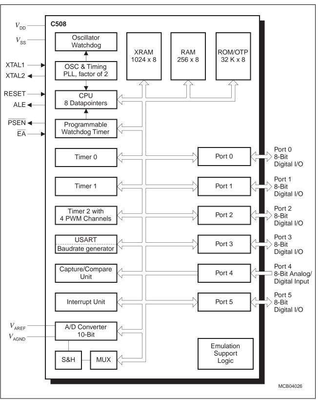
Figure 5 Block Diagram of the C508
