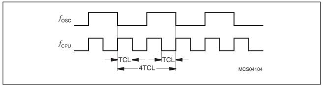
Figure 33 Relationship between Oscillator and CPU Clock
