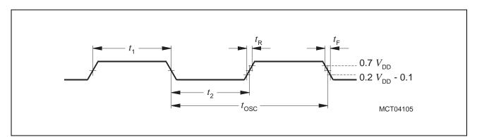
Figure 37 External Clock Drive on XTAL1
