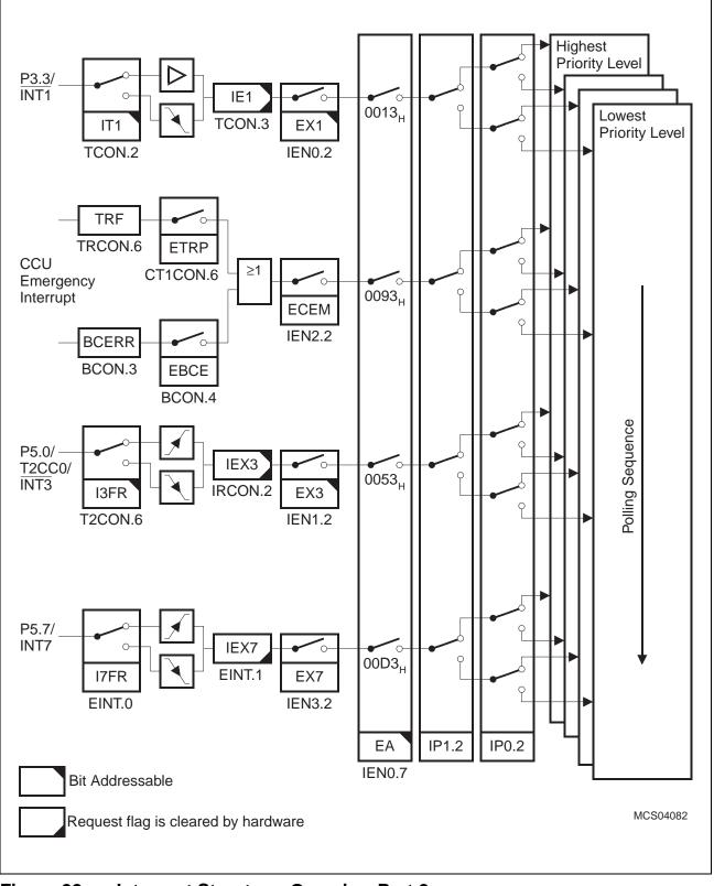
Figure 22 Interrupt Structure, Overview Part 2
