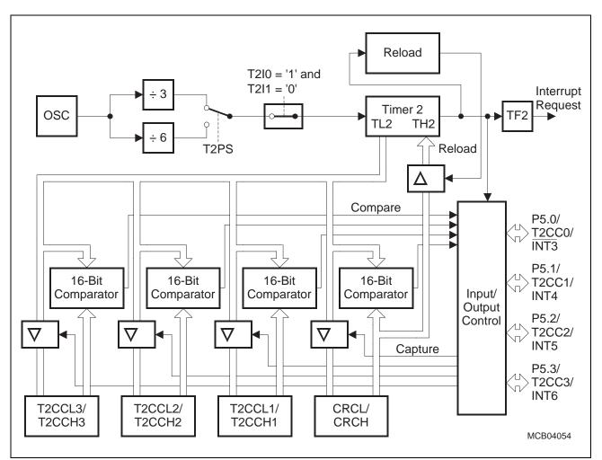
Figure 11 Timer 2 Block Diagram
