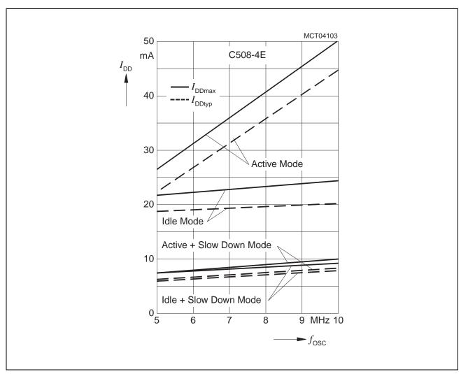
Figure 32 I<sub>DD</sub> Diagram
