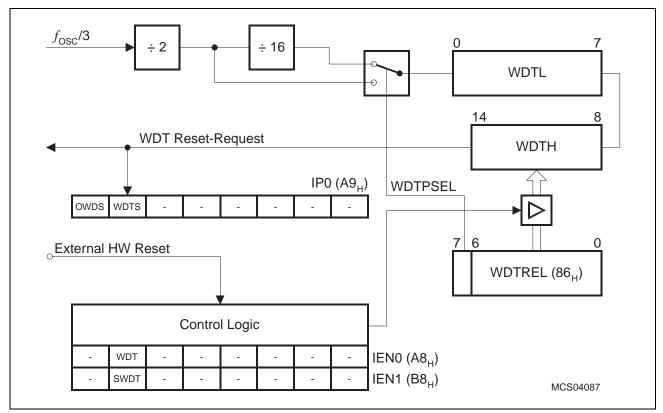
Figure 26 Block Diagram of the Programmable Watchdog Timer
