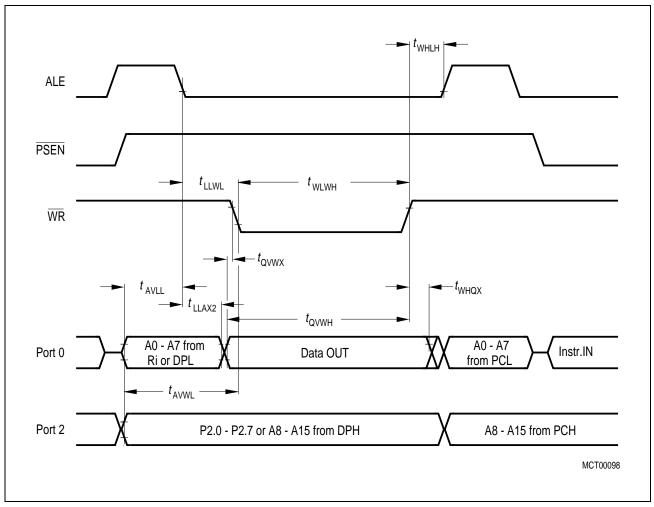
Figure 36 Data Memory Write Cycle
