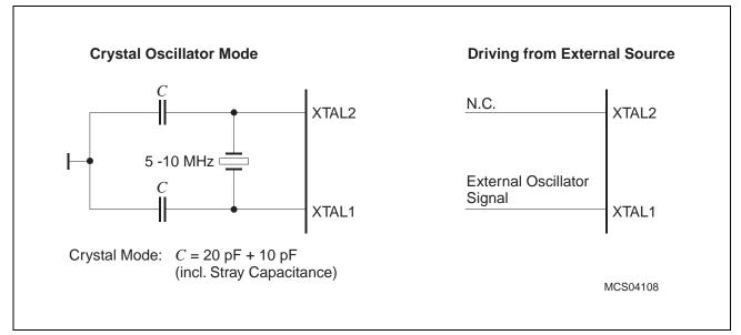
Figure 46 Recommended Oscillator Circuits for Crystal Oscillator
