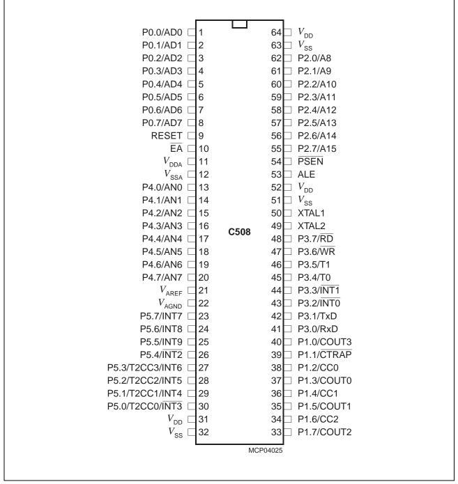
Figure 4Pin Configuration for P-SDIP-64-2 Package (top view)
