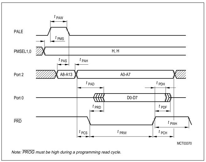
Figure 39 Verify Code Byte - Read Cycle Timing
