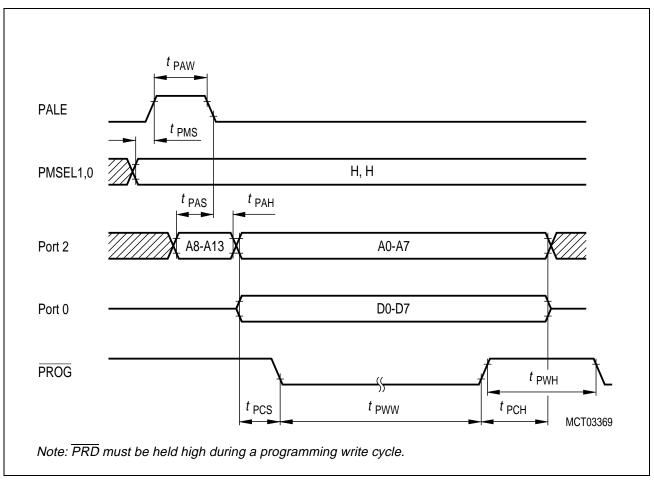
Figure 38 Programming Code Byte - Write Cycle Timing
