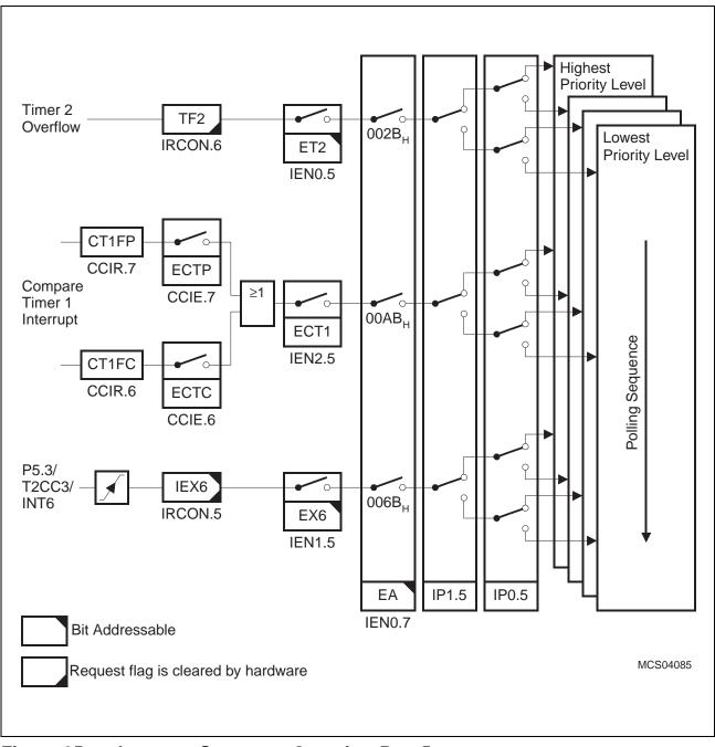
Figure 25Interrupt Structure, Overview Part 5
