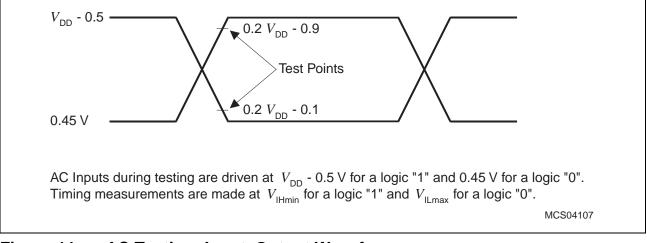
Figure 44 AC Testing: Input, Output Waveforms
