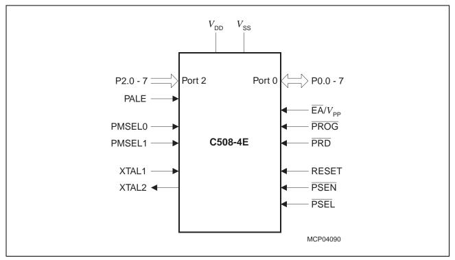
Figure 28 Programming Mode Configuration
