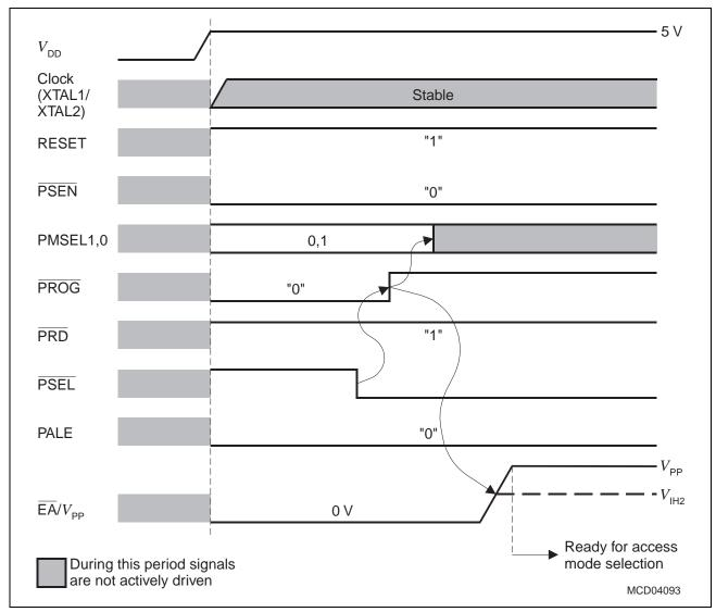
Figure 31Basic Programming Mode Selection
