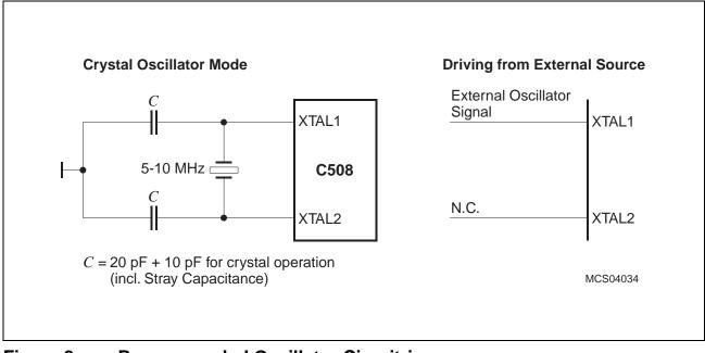
Figure 8 Recommended Oscillator Circuitries
